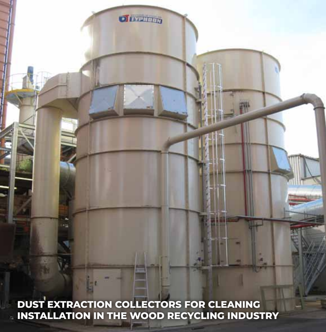
PNEUMATIC CONVEYING OF WOOD CHIPS WITH CYCLO-FILTER
